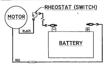
Refer to the electrical schematic above. Strip approximately 1/2" of insulation from the ends of the wires and crimp on the terminals as shown. For best results, solder the connections using electrical grade solder. Attach the wires to the rheostat switch and battery as shown.
